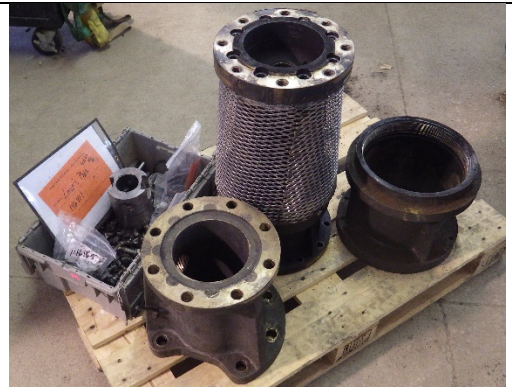
Suction and adaptor in good condition
