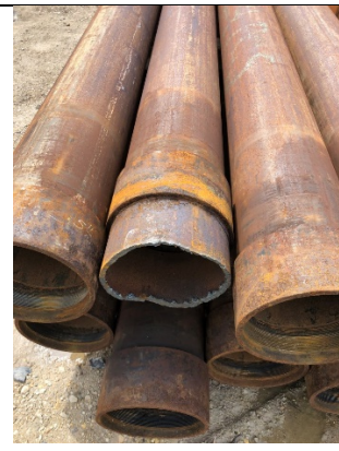
Threads were damaged from original install and 3 joints needed cutting
