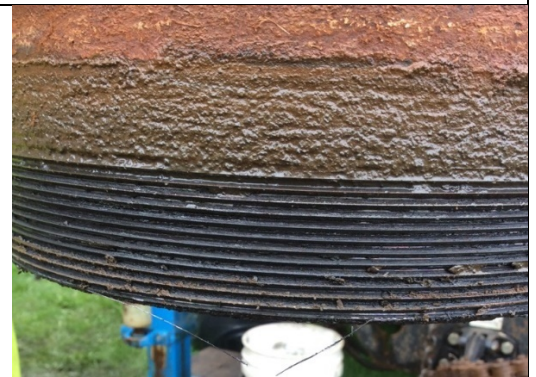
Washed out threads which cannot engage
