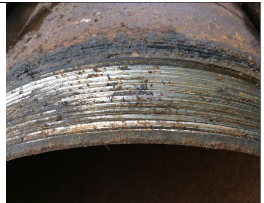
Washed out threads and very worn
