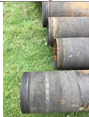
Threads were damaged from original install and 3 joints needed cutting
