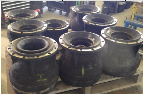
Bowl castings are in overall good condition
